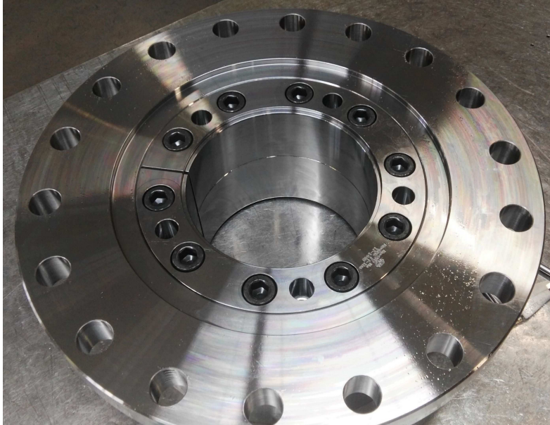
Figure 10. Re-assembling of each coupling half after step 11
