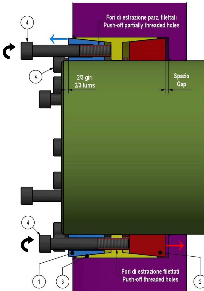
Fig. 2. Disengagement of thrust rings and positioning of Locking Assembly.
